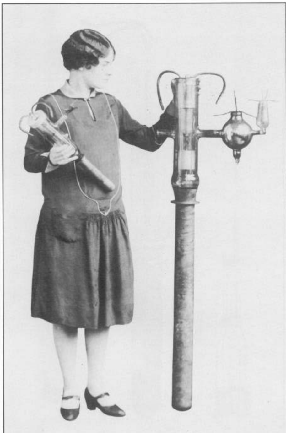
Fig. 11. The 100-kW water-cooled tube is the UV-862 at its stage of development in December, 1926. The rightmost appendage is a gas-gettering pump to maintain good vacuum in the earlier tubes. The small tube being held is the UV-207, the first of the water-cooled "metal" line.
