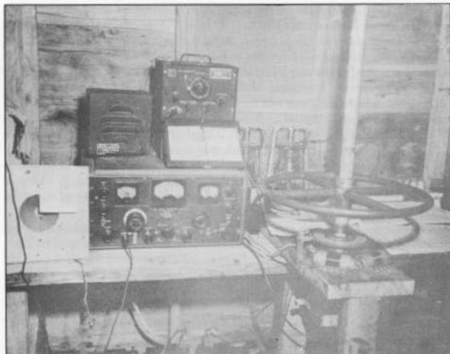
Interior of Adcock DF with BC-221 frequency meter and Hallicrafters SX-28 receiver. Spartan surroundings: storage batteries for power, oil lamps.
