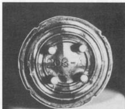
Molded marking on the base of a 203A/VT-1.
