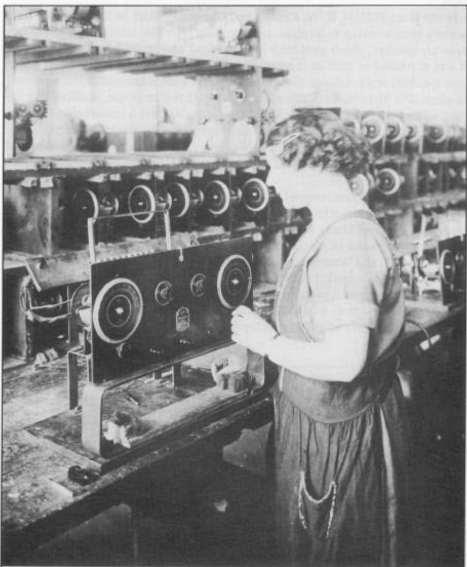
Fig. 6. A panel testing setup for the Radiola Superheterodyne. Photographed July 1, 1924.
